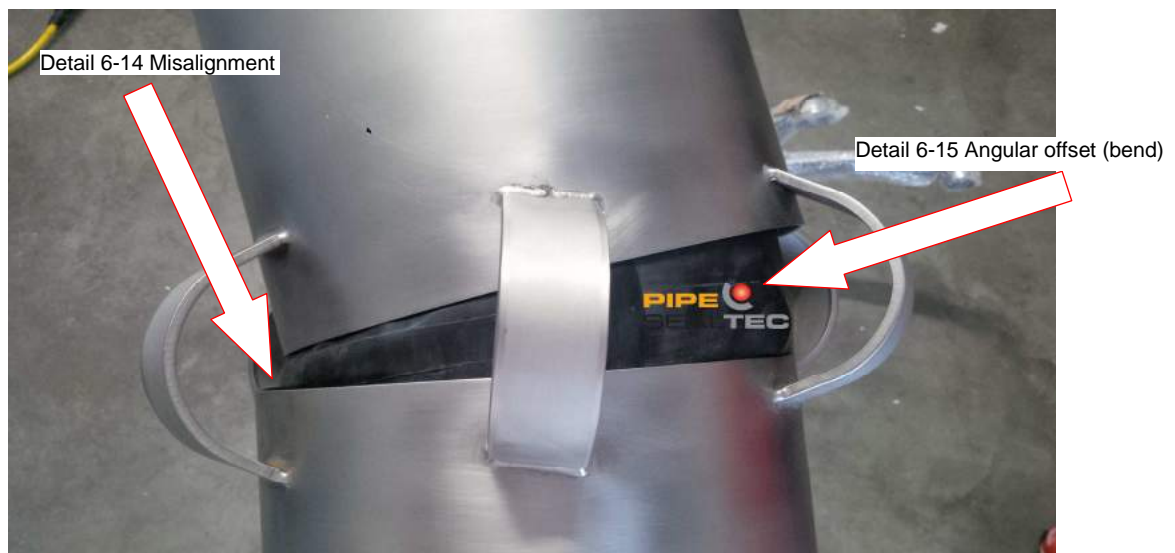
Figure 6-60 Test set-up axial and radial change of direction (angular offset and misalignment)
