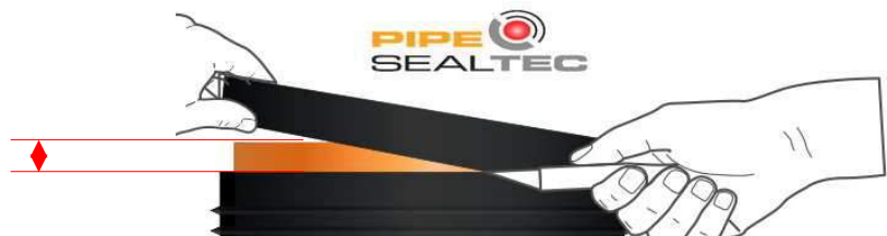
Sizing 6-1 Distance rubber – sleeve border min. 0.5cm -1.0cm
