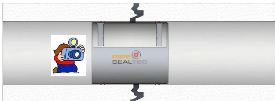
Figure 6-44 damaged area rehabilitated with Pipe-Seal sleeve - Documentation
