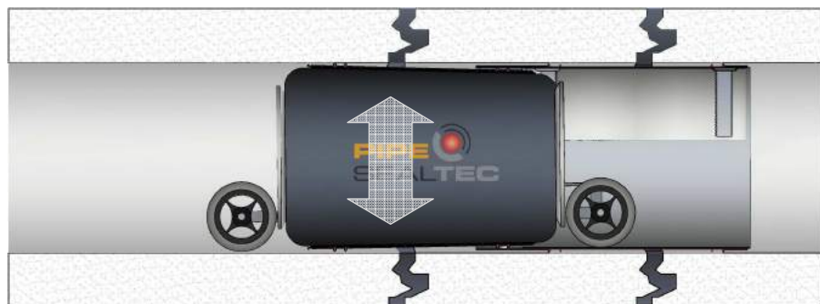
Figure 6-52 Expansion at the place of installation – Mounting the end sleeve
