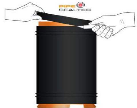
Figure 6-31 circumferential cut of overlapping rubber
