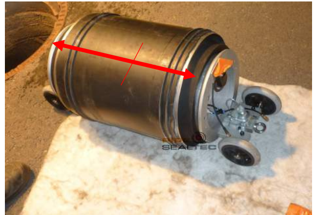
Figure 6-34 positioning the prepared stainless steel sleeve on the packer
