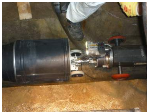
Figure 6-9 Mounting system Robot unit / displacement packer and robot adaptor
