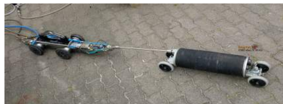
Figure 6-8 Mounting system TV-unit / displacement packer and connecting rod
