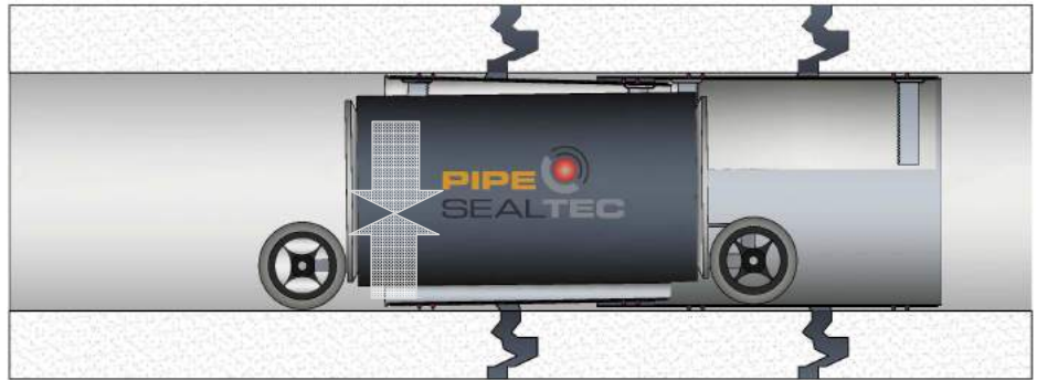
Figure 6-53 Pressure relief completed before removing the packer
