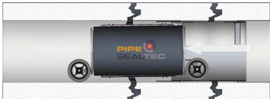
Figure 6-49 Mounting direction of another sleeve in a serial mounting
